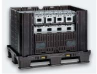
MegaPack JUMBO with HDPE interlayers to accommodate cylinder heads.
