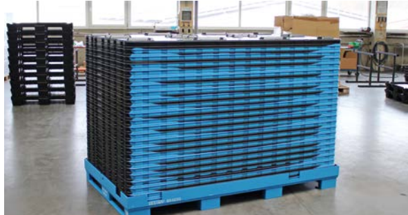
Load carrier with steel pallet and plastic lid for transporting cooling plates for battery cases (2244 x 1324 x 1468 mm).
