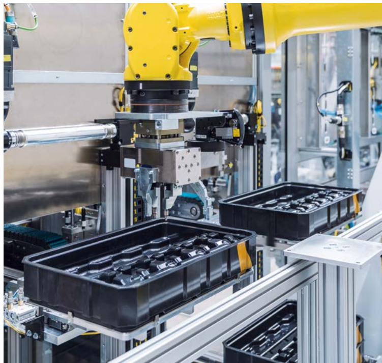
Container in 600 x 400 mm format for HDP trays and lids. Use in an automated assembly facility.
