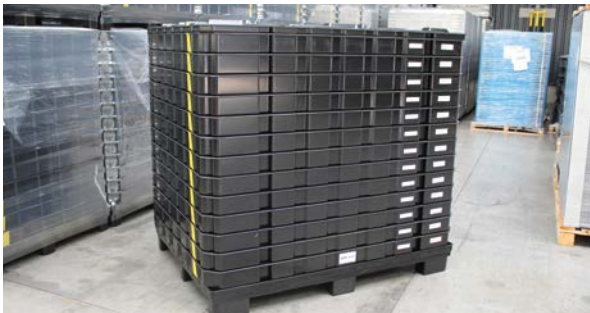
Packaging unit consisting of pallet, containers and lid for panoramic glass roofs (1466 x 1231 x 1473 mm).
